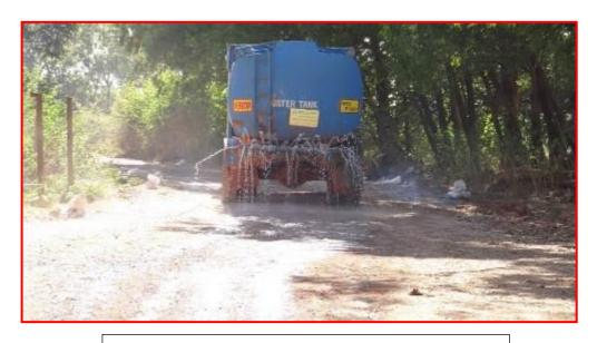
Water Tanker used for dust suppression.
