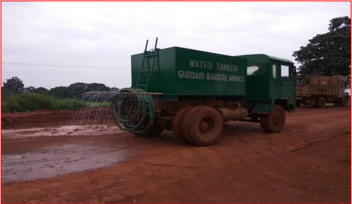
Water Tanker for dust suppression
