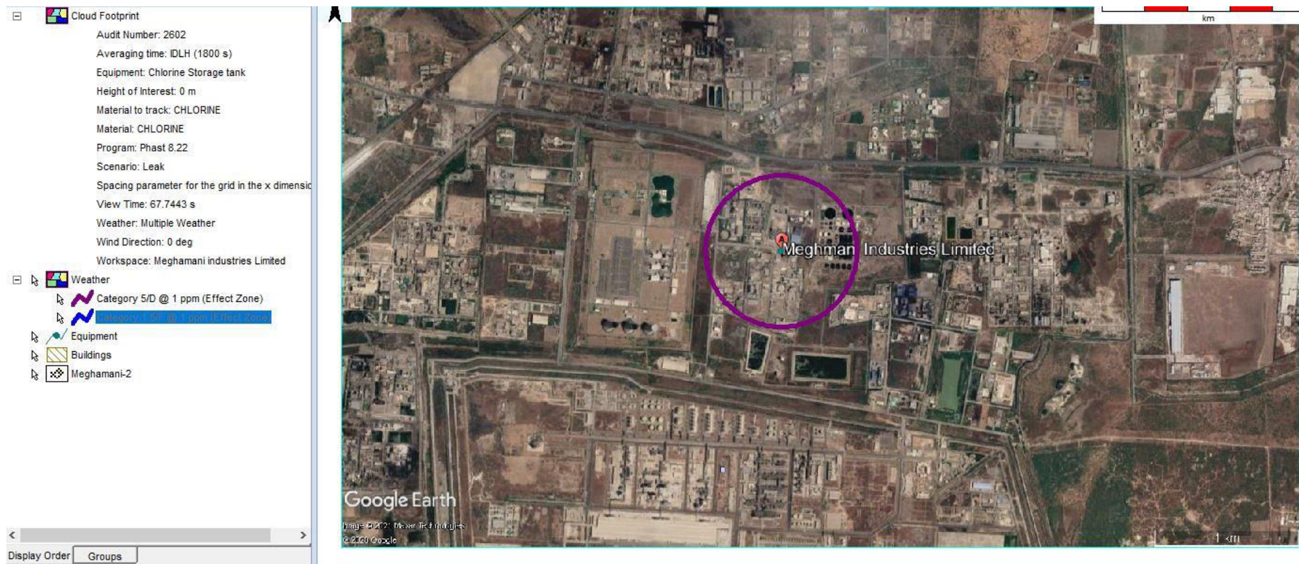
Figure 20: Cloud Foot Print of Leakage from Chlorine storage tank at 5D weather condition
