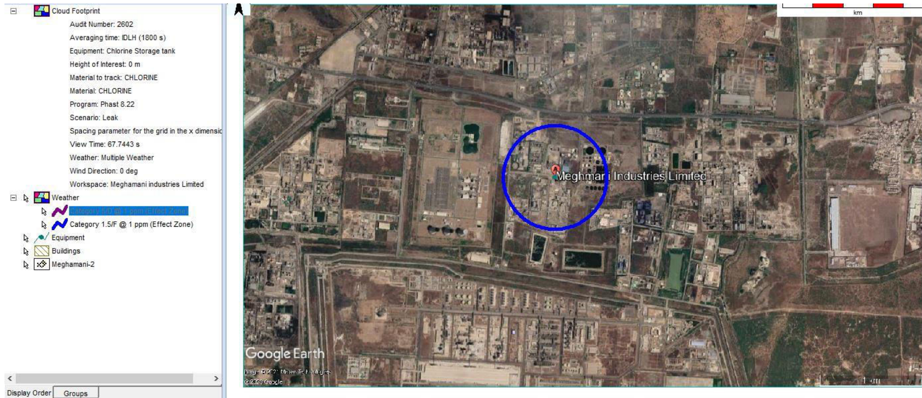
Figure 19: Cloud Foot Print of Leakage from Chlorine storage tank at 1.5F weather condition
