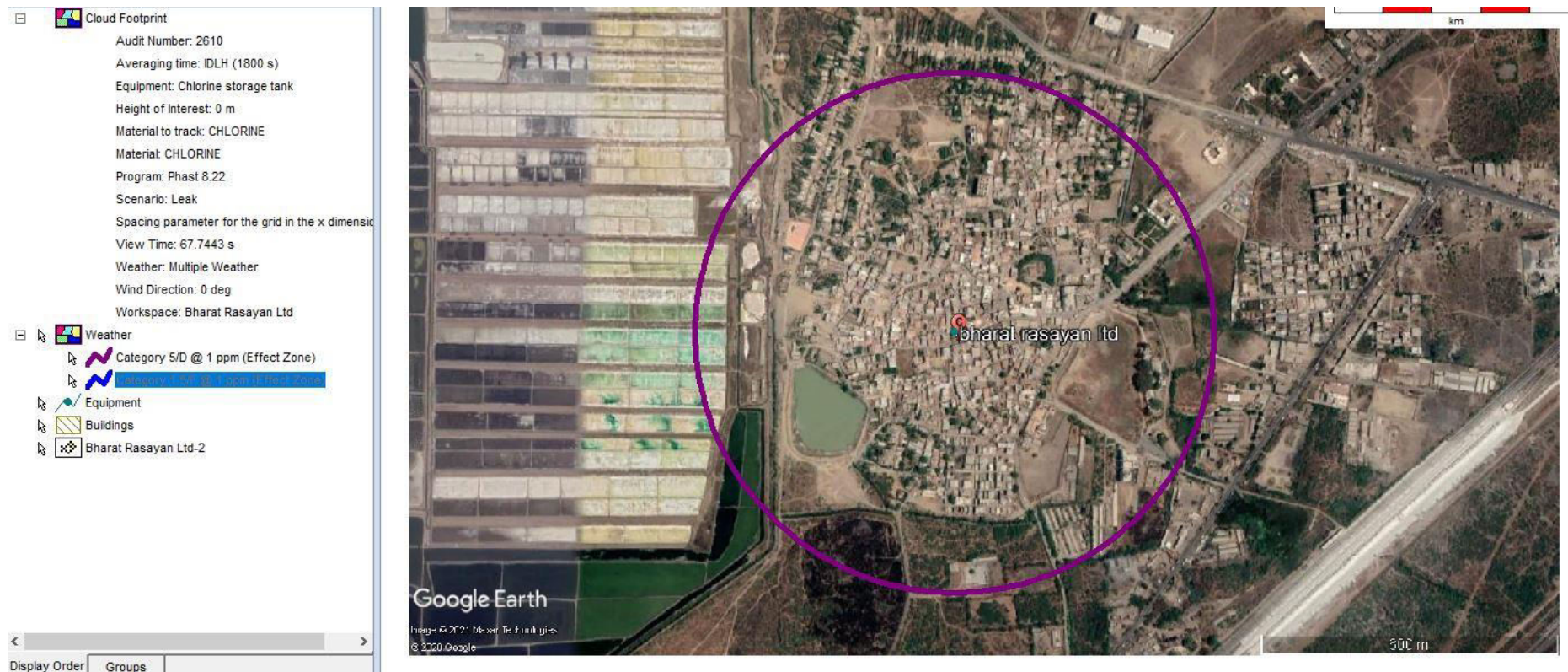
Figure 8: Cloud Foot Print of Leakage from Chlorine storage tank at 5D weather condition
