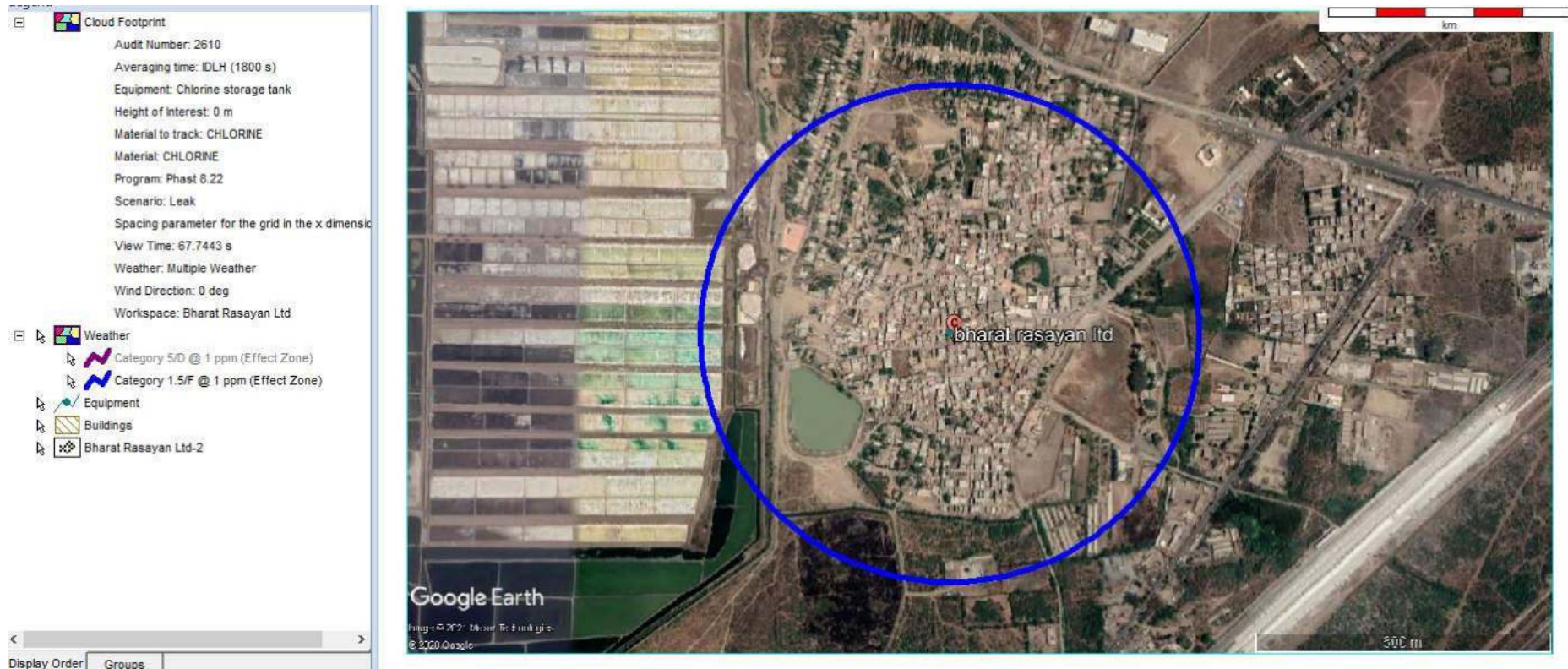
Figure 7: Cloud Foot Print of Leakage from Chlorine storage tank at 1.5F weather condition
