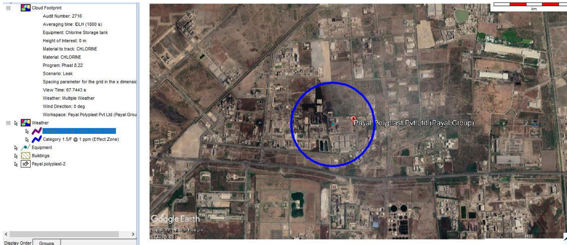
Figure 23: Cloud Foot Print of Leakage from Chlorine storage tank at 1.5F weather condition
