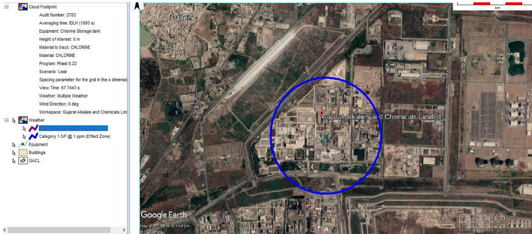
Figure 11: Cloud Foot Print of Leakage from Chlorine storage tank at 1.5F weather condition
