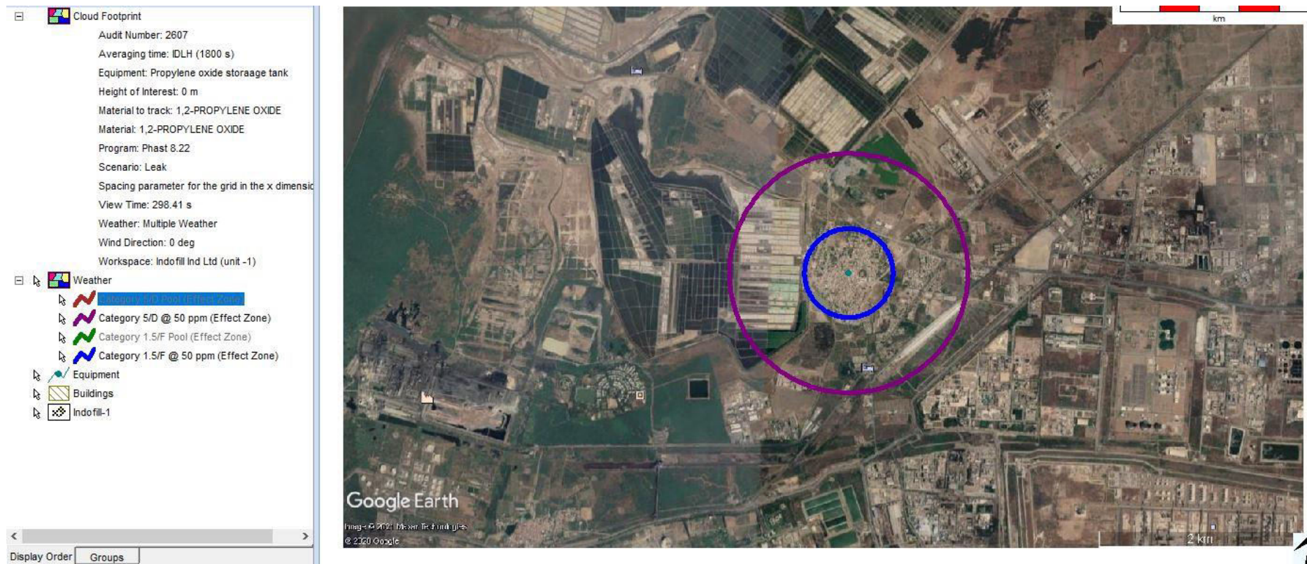
Figure 2: Cloud Foot Print of Leakage from Proylene Oxide storage tank
