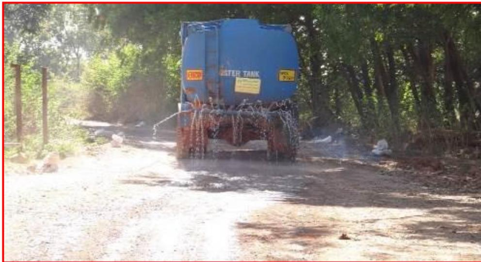
Water Tanker used for dust suppression.
