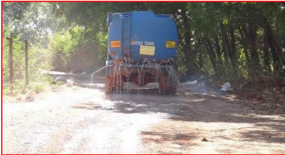
Water Tanker used for dust suppression.
