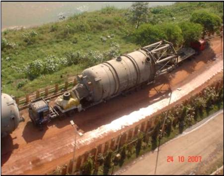
Pressure decanter recd. at site
