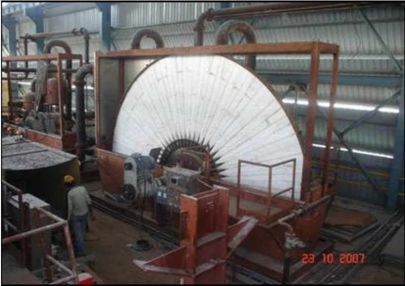
Fine seed disc filter being assembled
