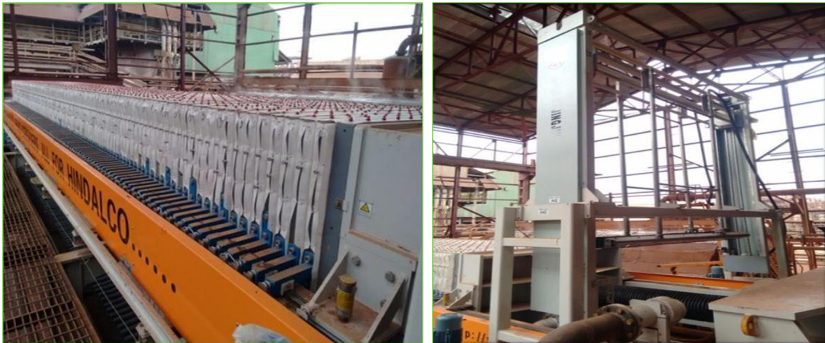
Photo: Pressure Filter
