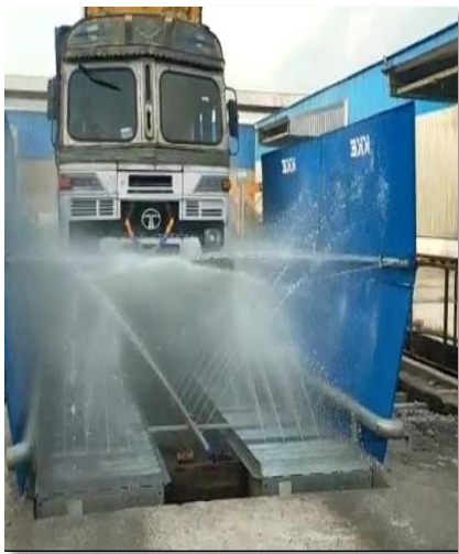
Wheel washing system
