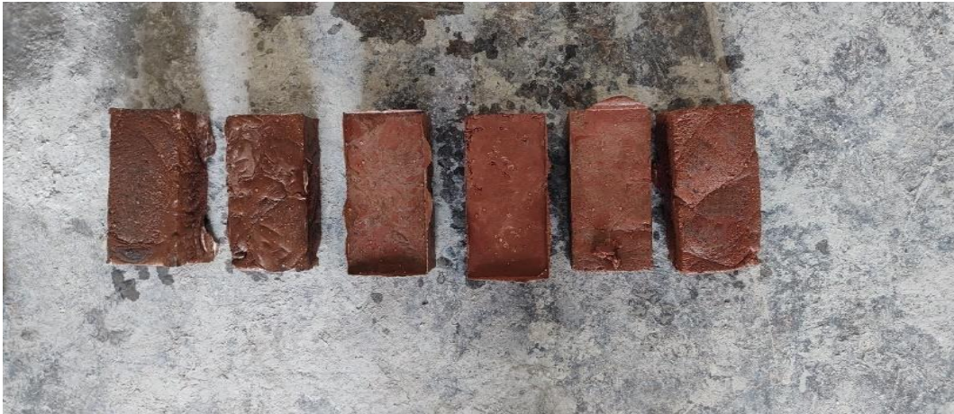
Polymer composite brick manufactured at Belagavi
