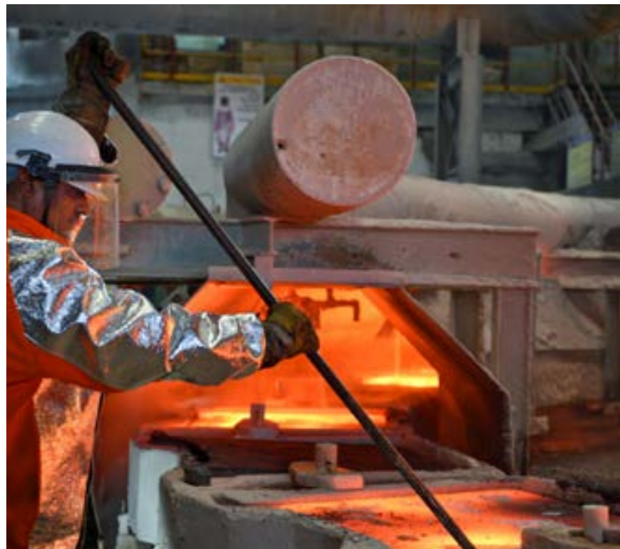
Smelter 1- Anode casting area at Birla Copper, Dahej
